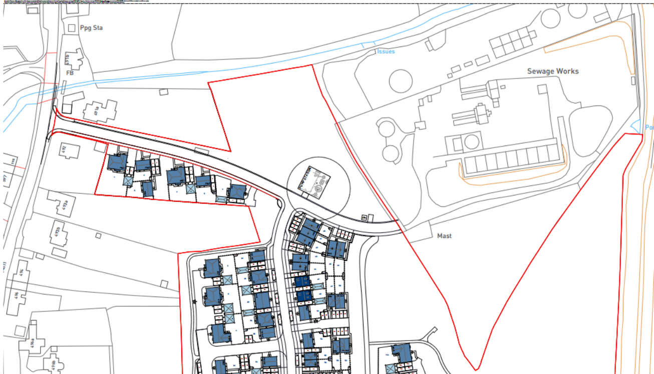
Partial plan extract using the Building Heights Plan showing the new vehicular access to the sewage treatment works.
